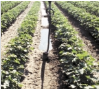
Figure 6. LEPA center pivot with drag sock.
