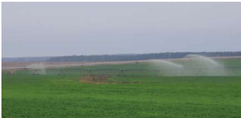
Highbrighton/Barrington Dairies recently faced a challenge of having to avoid applying effluent near a drainage ditch and buffer area. As shown here, the sprinkler guns on the Highbrighton/Barrington pivot turn off as they approach the drainage ditch.
