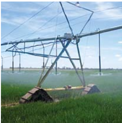
Lindsay's Z-TRAX tracking system provides improved flotation and reduced rutting on Protheroe's pivot irrigated rice.
