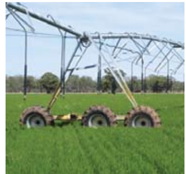
The Zimmatic rice pivot on Brian Protheroe's farm in Australia includes three-wheel drive tubes for improved traction and flotation and to eliminate pivot bogging.
