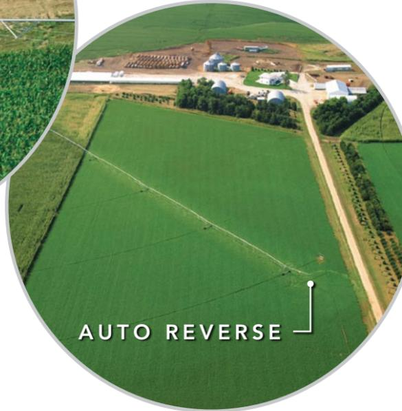
The FieldPLUS pivoting joint can be positioned at nearly any tower. Upon reaching a barricade, the tower automatically stops while the outer spans continue to operate. The auto shutdown-auto reverse allows the outer spans to return to the home position.
