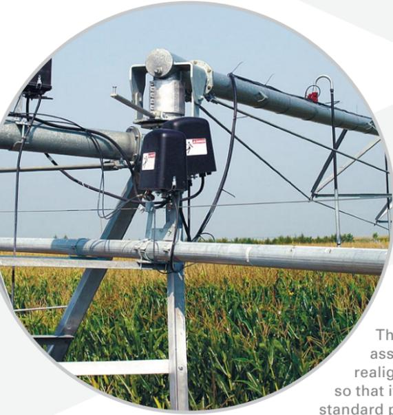
The pivoting joint assembly automatically realigns the entire system so that it can function as a standard pivot.
